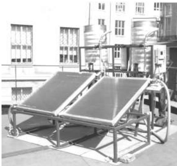
**Figure 5** – Photograph of the test rig.
